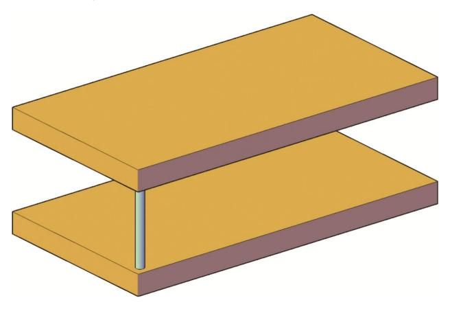
3. Create a 3D rectangular array of three rows, five columns, and two levels. Make the distance between rows and columns 10', and the distance between levels 12'-8". Create an associative array.
